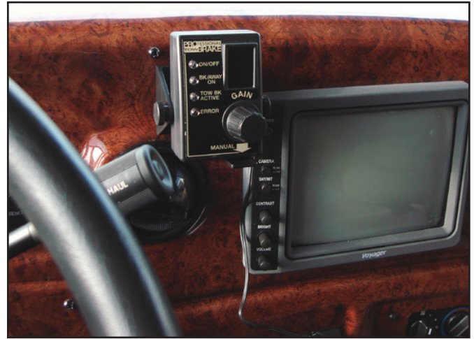
RF in-coach controller mounted on dashboard
